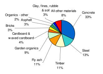
Figure E-1 Composition of recovered materials (by weight), SA 2006–07
