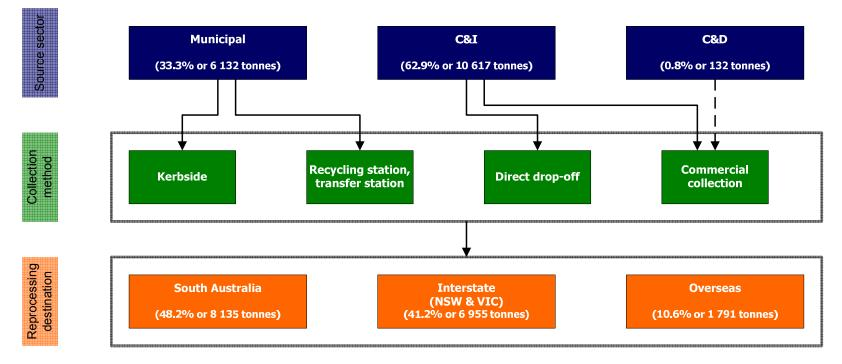
Figure 5-21 Flow of plastics reprocessing, SA 2006
